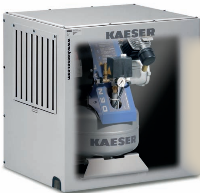
The use of a sound enclosure significantly reduces a dental compressor's sound levels. Depending on model, sound pressure levels of 60, or even 52 dB (A) can be achieved.
